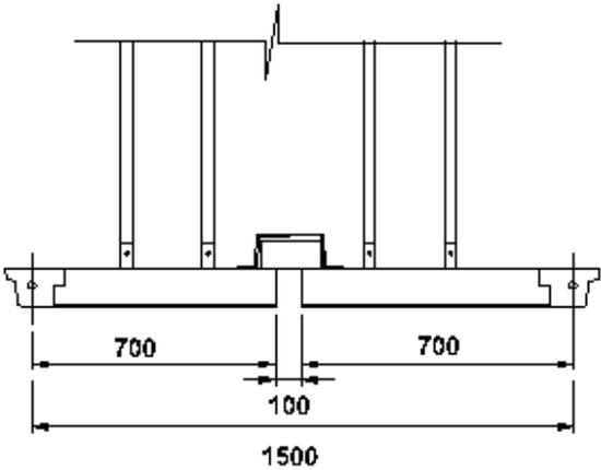
Figure 8. Plan view on cladding at settlement joint
