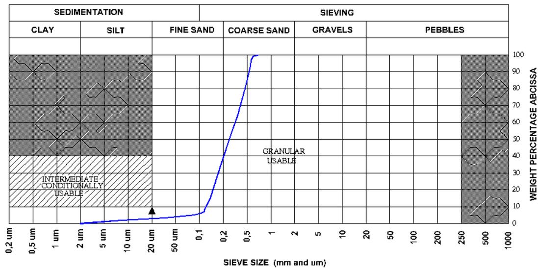
Figure 5. Backfill specification graph for Reinforced Earth®
